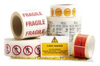
Pressure sensitive labels are made from label stock. Label stock is a multilayer laminate consisting of a face material or "facestock" (the surface of the label on which the text will be printed), an adhesive, a silicon coating (which allows an easy release of the face material from the base material), and the base material or "release liner" (which protects the adhesive). <sup>1</sup>
