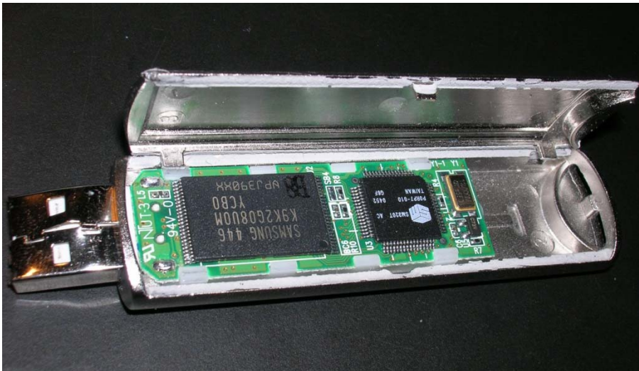
Flash Memory System showing flash memory chip (left) on circuit board with controller (right) within USB flash memory system product casing (credit: http://upload.wikimedia.org/wikipedia/commons/8/8c/USB_Drive_Open.jpg )
